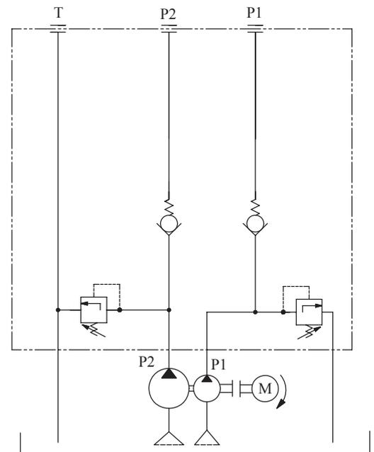
The W85D series power pack is designed for applications that need two independent hydraulic power supply, but only use a single D.C. motor.
